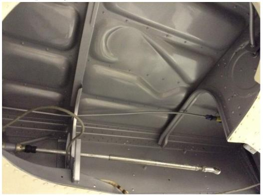
(https://francomarquis.wordpress.com/gear-inspection-ad-77-13-21-part-a/gears-193/) Time to do the well's rear closure plate and its edge protection. Note the main gear bump pad is being glued in place. Sure the exterior paint will need some attention... eventually.
