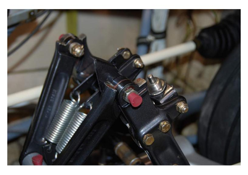
The up limit switch will also require adjustment and the SM describes the method to do that. The transmission can be re-connected and the gears swung. The gear doors that can now be re-rigged as per the SM.
