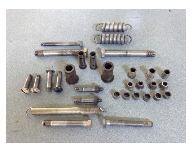
Bushing removal and re-insertion as usual, heat with a propane torch to extract and a press bench to re-insert. Any diameter reaming done on a drillpress. Measurements to the sidebrace threads were done at a machine shop equipped to do such. Luckily were found within service limits. Also, I replaced the nosegear springs (487-292) as they were no longer showing the service tension (which I cannot find anymore...sorry)
