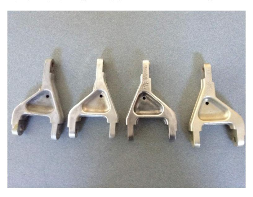
Then, steel parts are stripped with glass bead and then sent for cadmium plating.
