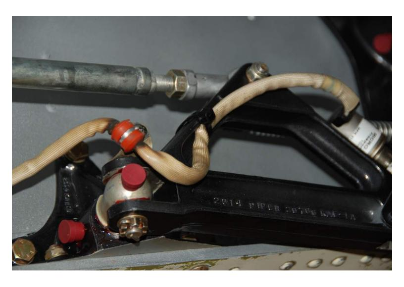
Main gears are anchored in place. There are a number of shims on these where the longitudinal movement is stopped. The existing sequence on my plane was wrong and a few trials were necessary to get it perfect.
