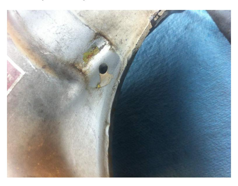
Landing gear doors tend to also take a beating. While I did the conduits, some time ago, I made the hinges tighter by drilling a #30 hole and inserting a 1/8 SS welding rod as the hinge pin. That made the door much stiffer and I did not pay much attention to them after that. However, stripping them led to discover other issues that needed attention. A few pictures are worth a proportional number of words on the quality of these repairs...
