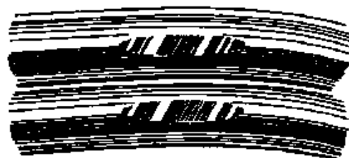
INDIVIDUAL OUTER WIRES WORN LESS THAN 40% (WORN AREAS INDIVIDUALLY DISTINGUISHABLE)
