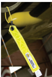
The PSR-BFS1007 is a remove before flight streamer used to bring attention during the preflight inspection
