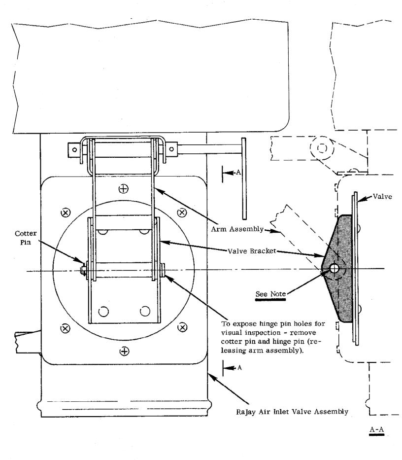
NOTE - Inspect RaJay Alternate Air Inlet Valve Bracket hinge pin holes (2) for wear elongation exceeding 1/16 inch. Replace if required with new alternate air inlet valve and bracket assembly RaJay Part No. RJ0605-5/-71.
