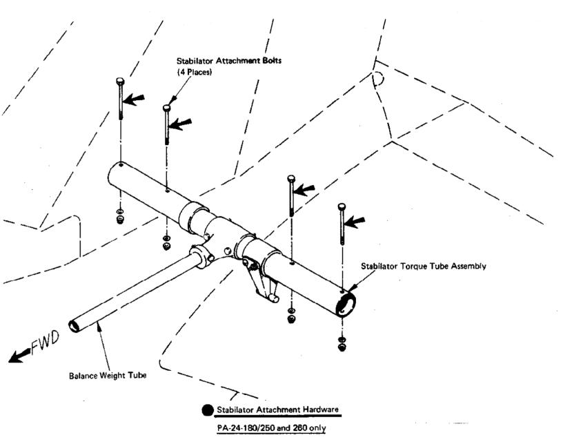
Bolt AN174-C32A P/N 502 329 (Corrosion Resistant) or Bolt AN174-32A P/N 402 329 (Non-Corrosion Resistant) Washer AN960-416L P/N 407 585
