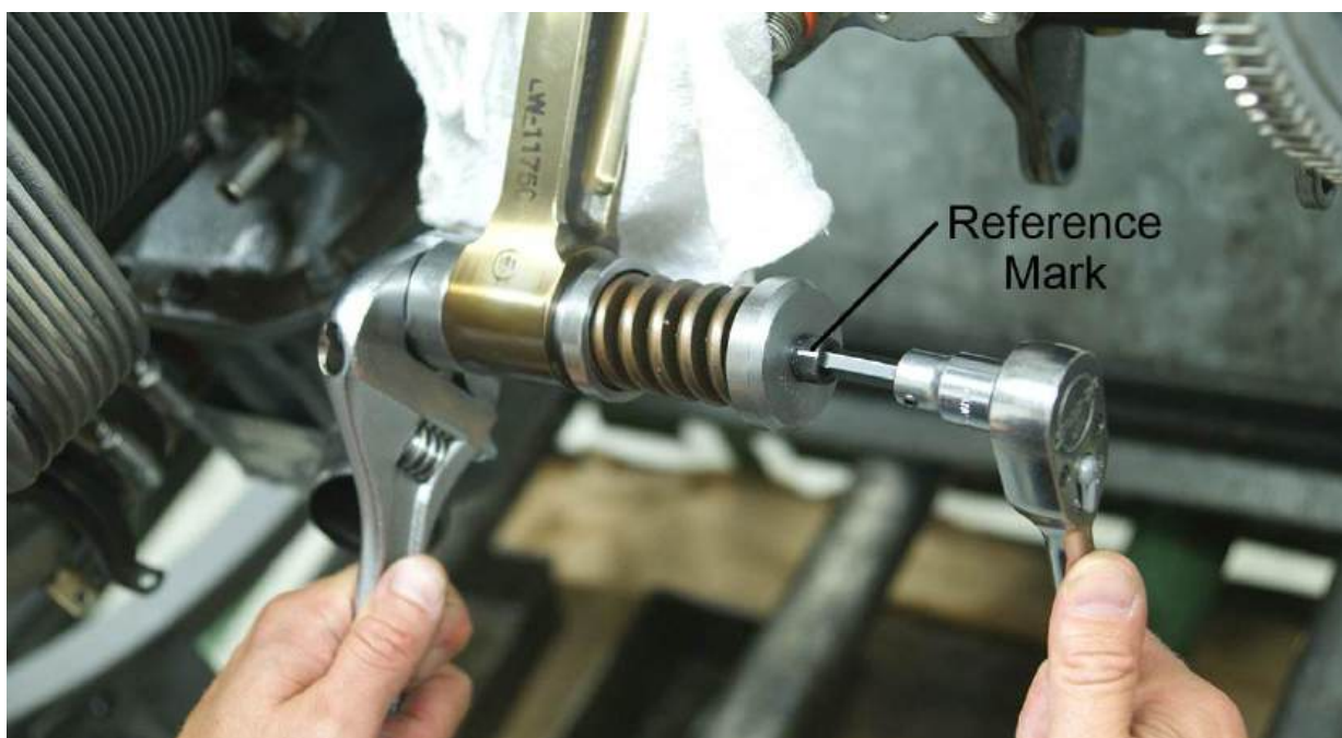
Figure 10 Turn the Bolt 6 Turns
